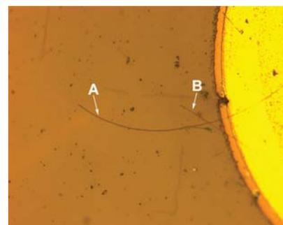
Micrograph of a complete nanowire LED with the end contact. The long nanowire (A) is about 110  $\mu\text{m}$  long, a shorter nanowire (B) crosses it. The bright circular section is the metal post from which the nanowires are aligned.
