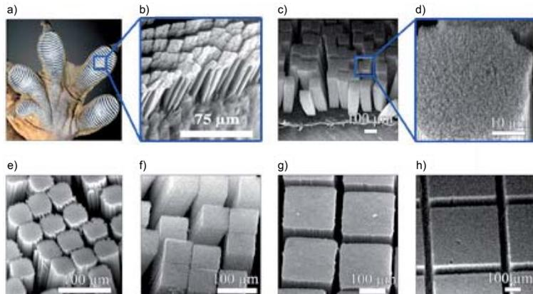
*Microfabricated aligned multiwalled carbon nanotube setae and spatulas. (a) Optical picture of gecko foot showing that the setae are arranged in many lobes along the foot. (b) SEM image of natural gecko setae terminating into thousands of smaller spatulas. (e–h) SEM images of synthetic setae of width (e) 50, (f) 100, (g) 250, and (h) 500  $\mu\text{m}$ . (c) Side views and (d) higher magnification SEM image of the 100  $\mu\text{m}$  setae (Image courtesy of the University of Akron).*
