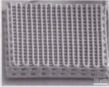
FIT TO PRINT A micronozzle secretes a stream of liquid polymers into a reservoir (top). As the computer-controlled nozzle moves across the surface, polymer streams coagulate into a three-dimensional structure (bottom).
